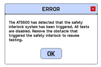
Should this error occur; check the operation and installation of the safety light curtain (see AT5600 user manual).
