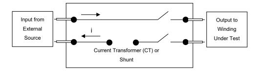
Test current flows from the external source into the fixture and out to the winding under test via an isolation relay.
