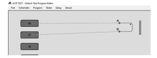
4, Add a VOCX test, with the same 19/A and 17/B nodes used for BOTH Energised and Measured terminals In this example we have programmed a sequence of 3 VOCX tests at 200, 400 and 600 Volts
