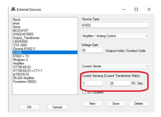
Current sense is much preferred over a voltage sense method, as the current sense method is much more accurate and more robust in an industrial environment.
