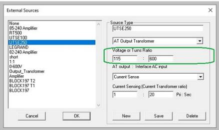
Note; Once this is set up, you will program the tests (VOCX, MAGX, WATX STRX) in the normal way, and enter your requested voltage that you require on the UUT. The AT will then apply and trim the input voltage to the transformer to get your required test signal for your UUT
